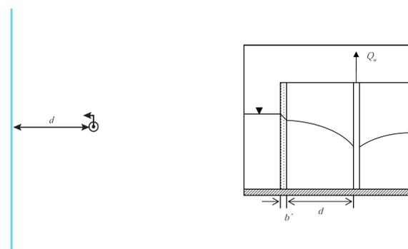
Figure 1. Hantush equation conceptual model.
