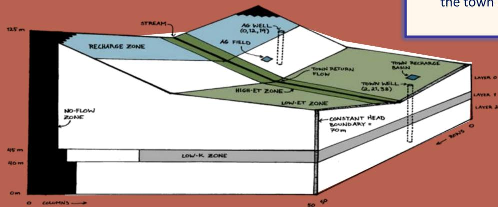
Figure 1 Schematic of the model aquifer. Courtesy of Chloé Fandel.
