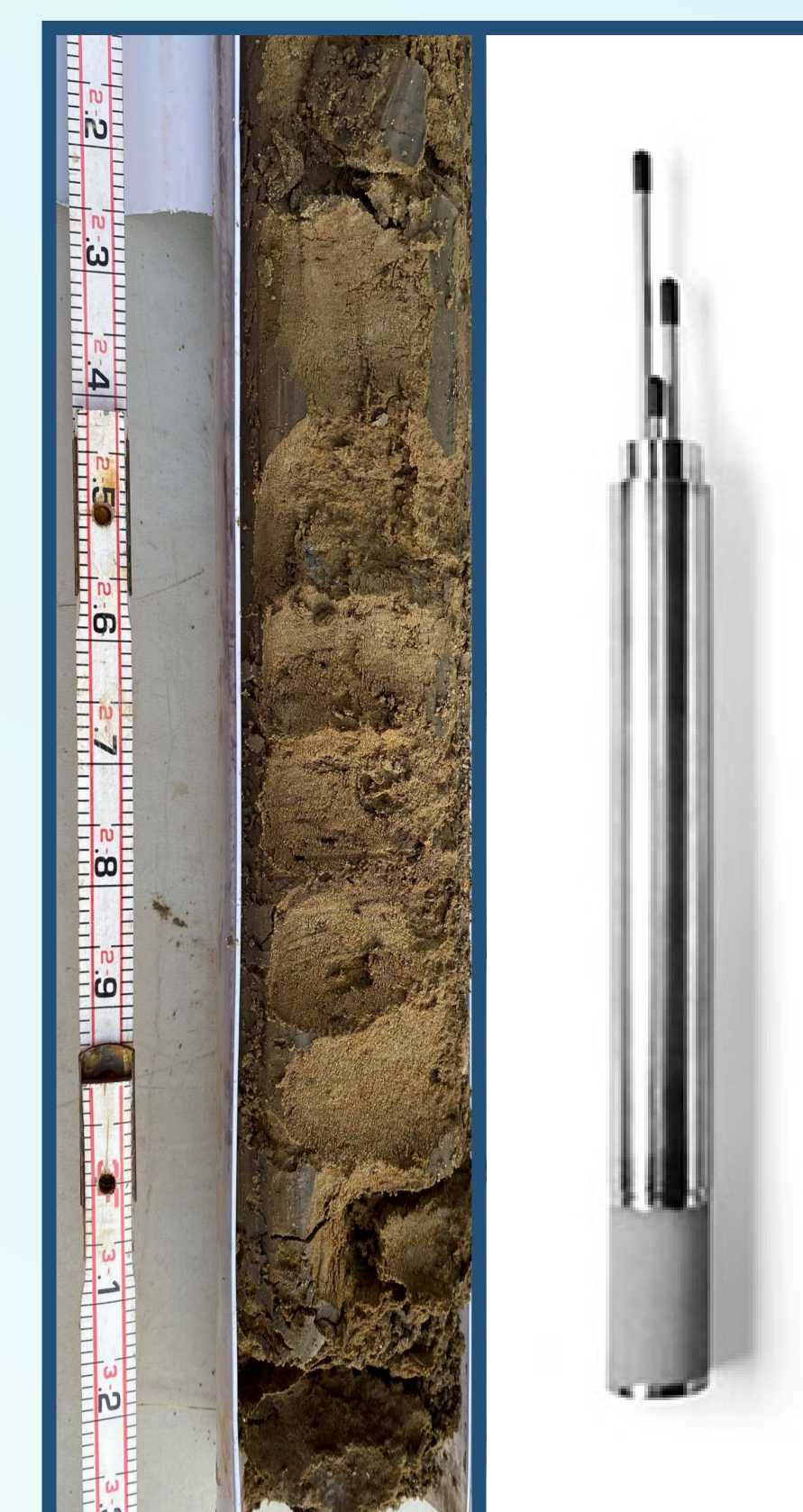
Example soil core and stainless steel lysimeter
